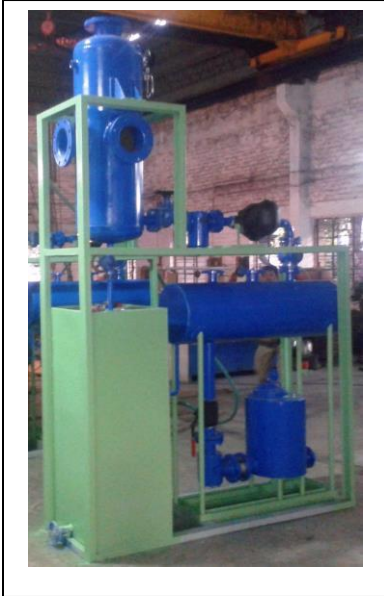
Single Pump Single Flash Vessel TRPS
