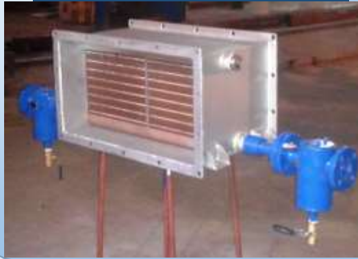
Heat Recovery From Exhaust Gas.
