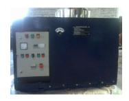
The "MICROSH" comes equipped with a PLC backed automated control system enabling a total user oriented flexibility for cycle time, sequence settings and final product size control.
