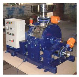
The "MICROSH" uses a specially developed revolutionary method of shredding instead of the traditional crushing method and thereby achieves better size reduction at a faster rate.
