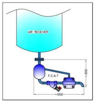
This is one time installation system which does not contain any instrumentation and hence has minimal maintenance challenges after it is installed. This strainer used in this system is with online cleaning facility hence no shutdown is needed to clean the strainer.
