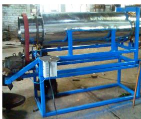
"BUNG WASHER" is a machine which, as the name suggests, washes the bungs with water and then rinses them before discharge.
